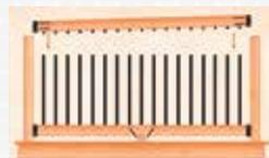
**6.** Start the top rail at an angle and insert the connectors into the balusters. Make sure your balusters are fully connected. Next install four #8X2" screws for each connector through the railing connectors into the posts. Please note that for spans more than 6" a foot block may be needed (recommended space between bottom rail and deck is 3-1/2" - check local codes).
