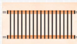
**5.** Finish mounting the balusters. Slide the Precision railing connectors on the rail ends ensuring the rail is fully seated in the connector. Next install two #8X2" screws through the connectors and into the rail ends.
