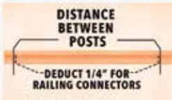
**2.** Using the measurement from the first step, subtract  $\frac{1}{2}$ " from the total measurement for railing connector. (Railing connectors are  $\frac{1}{4}$ " thick).
