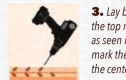
**3.** Lay bottom and top rails next to each other with the top rail flipped upside down. Position the rails as seen in image. Find the center of rails and lightly mark them. Measure out 5-1/2" from each side of the center line and lightly mark. The end spacing may vary. Set a combination square for center and lightly mark. Where the lines intersect will be the center of the Precision baluster connector.
