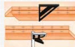
**2.** Using the measurement from Step 1- deduct  $\frac{1}{2}$ " from the total measurement for railing connectors. (Precision railing connectors are used for both level and stair applications) Then cut both the top and bottom rails to size.
