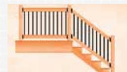
**6.** Start the Top Rail at an angle and then insert the connectors into the balusters until all of the balusters are in place. Ensure the balusters are fully connected. Connect top rail to post with four #8x2" screws through the railing connector and into the post on both sides.
