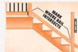
**1.** Lay bottom rail next to posts and mark them for angle. If the posts are plumb then the top rail should be the identical angle and length. Next cut the top and bottom stair rails at the correct angle.
