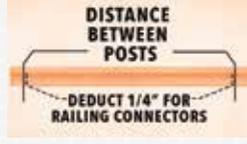
**2.** Using the measurement from Step 1, deduct  $\frac{1}{2}$ " from the total measurement for Precision railing connectors. Then cut both the top and bottom rails. (Precision railing connectors are  $\frac{1}{4}$ " thick).
