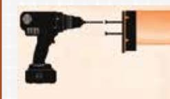
**3.** Slide the railing connectors on the rail ends and make sure rail is fully seated in the connector. Then install two #8X2" screws for each connector through the railing connectors and into the rail ends.
