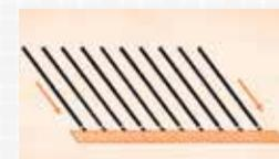
**4.** Insert a screw through the Precision baluster connector and install where the lines intersect (start vertically and then tilt screw to correct angle). The bottom and top baluster connectors will be facing in opposite directions.
